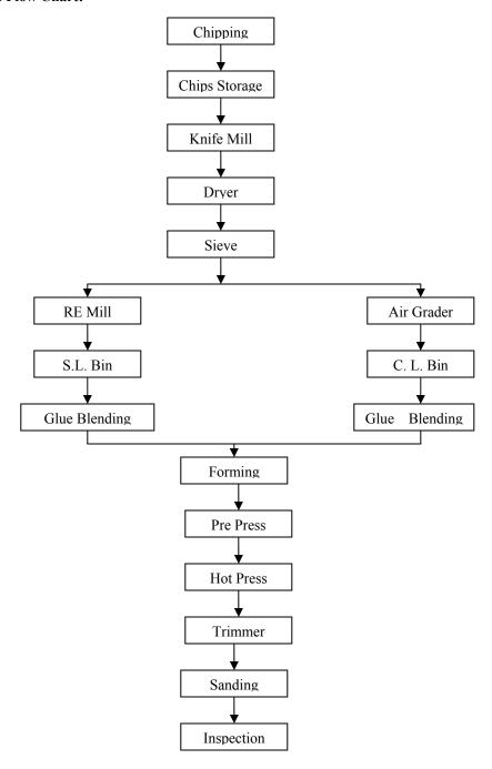
A brief on manufacturing process for production of plain particle board is described below.
