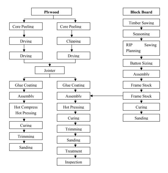
A brief on manufacturing process for production of plywood & block board is given below.
