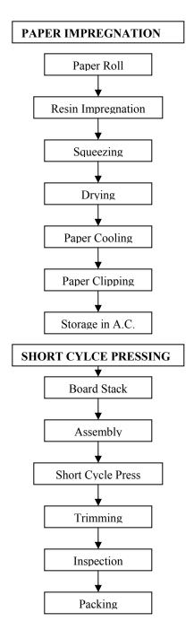
A brief on manufacturing process for production of pre laminated particle board is described below.
